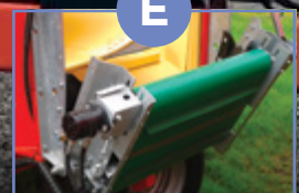
E Discharge Elevator Hydraulic discharge conveyors can be fitted to side door model vertical feeders to allow feed into bunkers.
