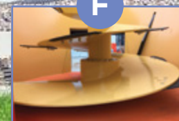
Mixing Auger Two vertical 15mm heavy duty augers to ensure perfect blend.
